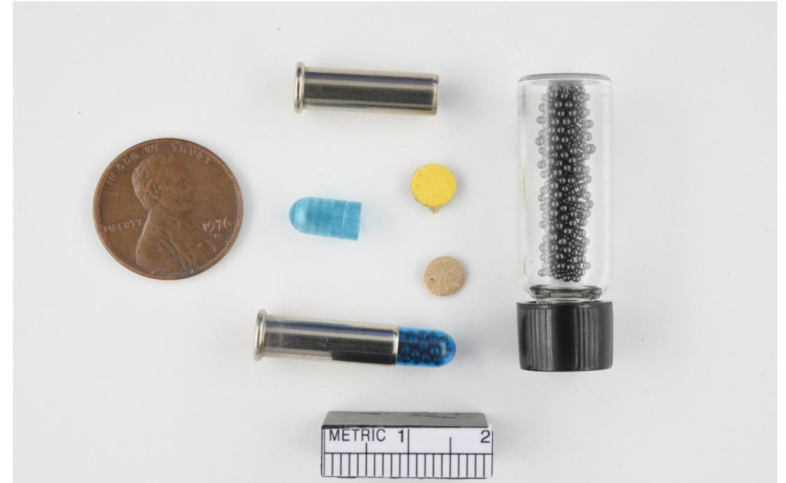
Example of small caliber (.22) snake shot ammunition broken into components including the plastic cap, shot, and small cardboard wads. Photo provided by Dr. Reade Quinton, Mayo Clinic Rochester.
